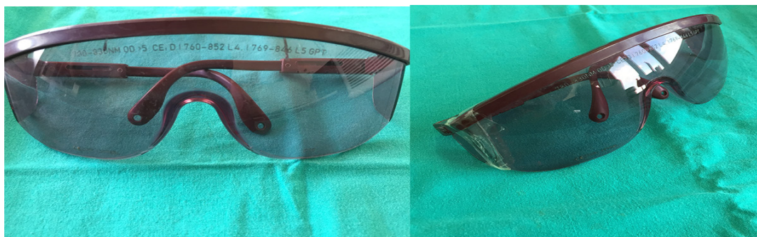
Figure 4. Goggles with visible scratches on the surface (left) or those which are broken (right) should not be used as they are unable to provide sufficient protection.
