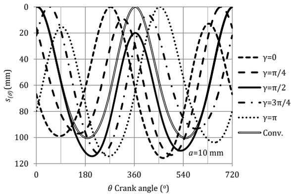
Fig. 8. Effect of  $\gamma$  angle on piston movement characteristics
