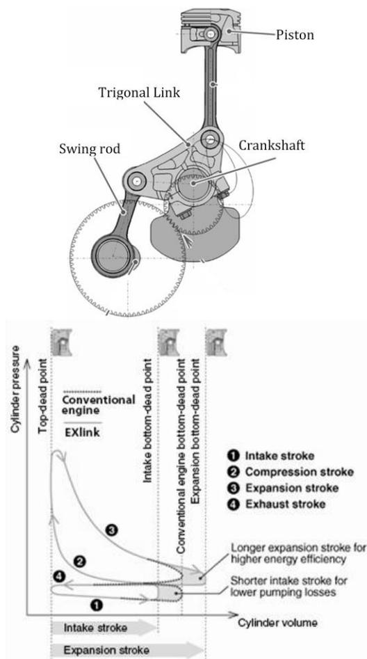
Fig. 1. Honda EXLink (Extended expansion linkage) engine [3]
