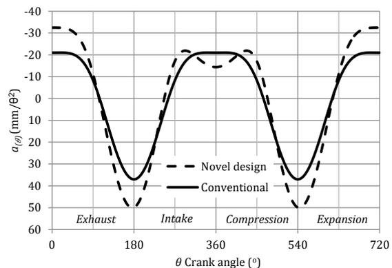
Fig. 11. Change of  $a_{(\theta)}$  according to  $\theta$
