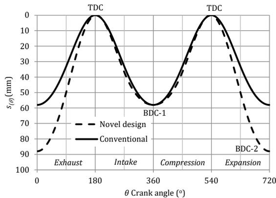
Fig. 9. Change of  $s_{(\theta)}$  according to  $\theta$
