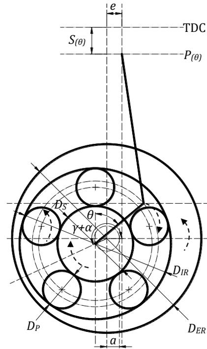
Fig. 4. Position of the crank-conrod mechanism
