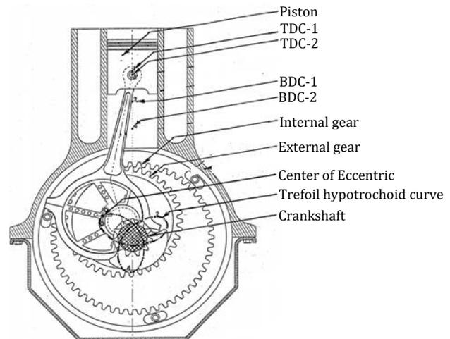
Fig. 2. Atkinson cycle engine using planetary gear system [18]
