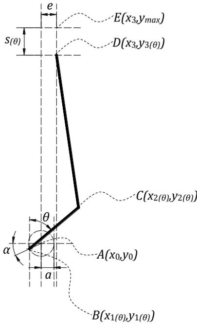
Fig. 5. Nomenclature of critical motion points in crank-conrod mechanism.
