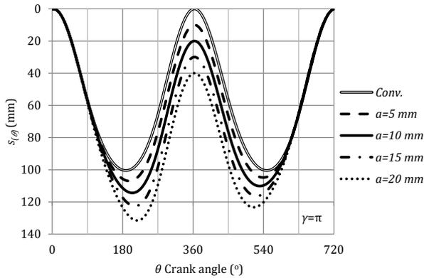
Fig. 7. Effect of central offset ( $a$ ) on piston path
