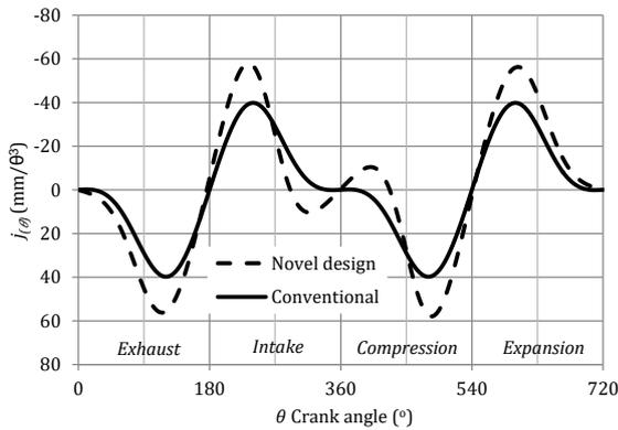
Fig. 12. Change of  $j(\theta)$  according to  $\theta$
