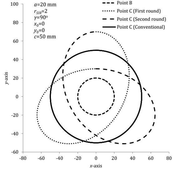
Fig. 6. The trefoil path of point *C*
