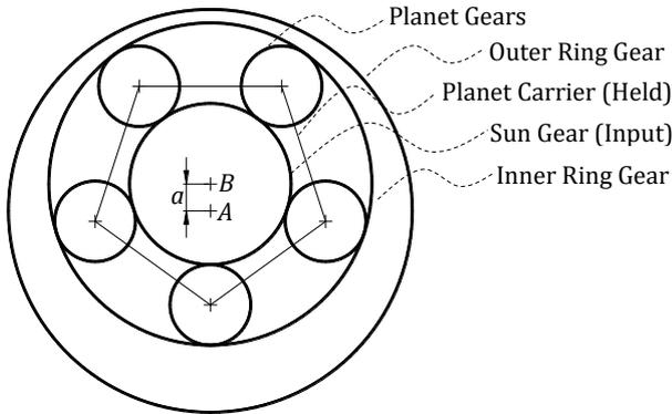
Fig. 3. Designed planetary gear mechanism
