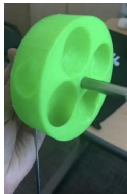
Figure 6. The origami inspired rotor design 3D print example.
