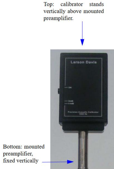
Figure 6. Microphone calibration by Larson Davis CAL200
