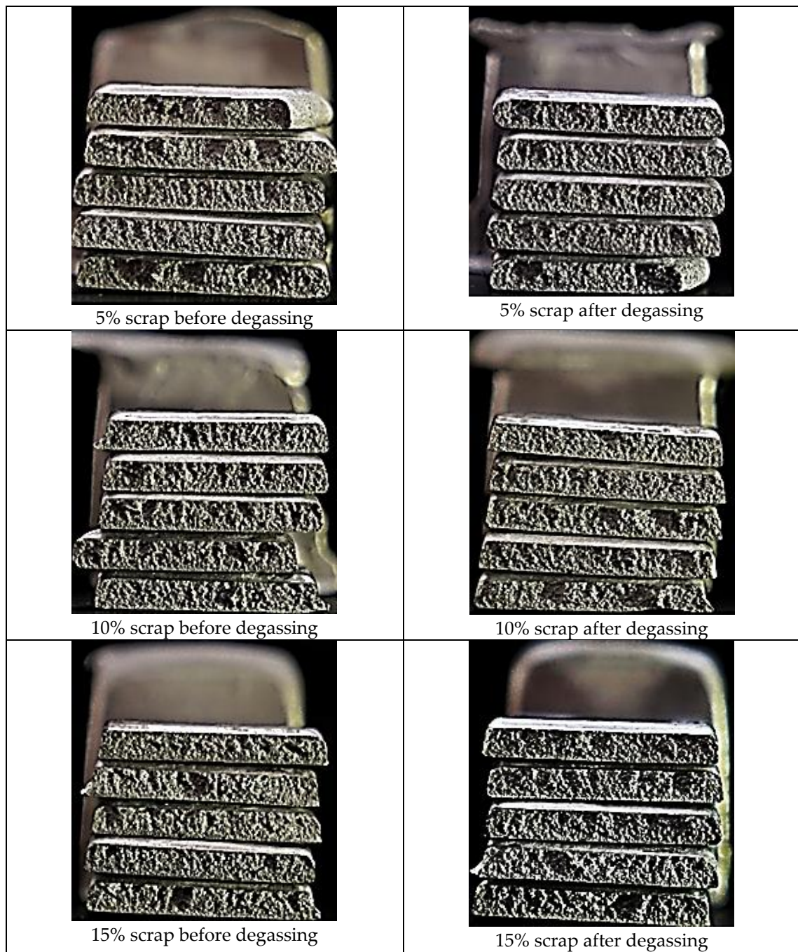
Figure 6. K-mold test specimens with different scrap ratios.
