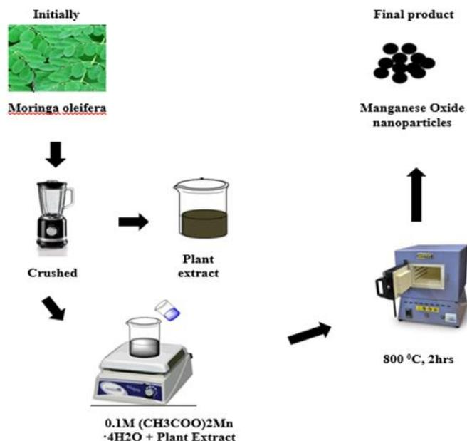
Figure 2. The green synthesis of MnO NPs
