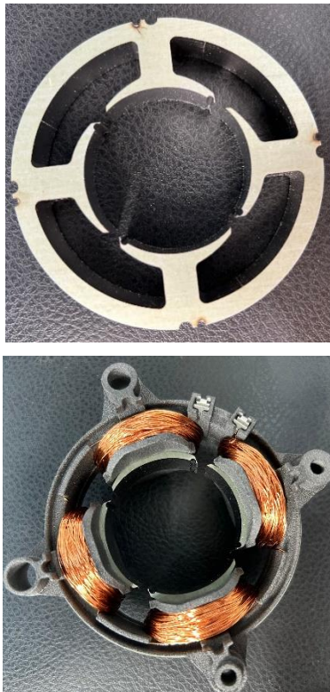
Figure 7. Notched stator in its stacked and wound state
