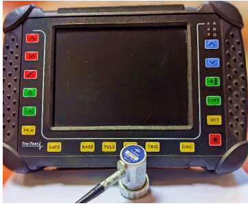
Figure 4. Ultrasonic testing device and probe used
