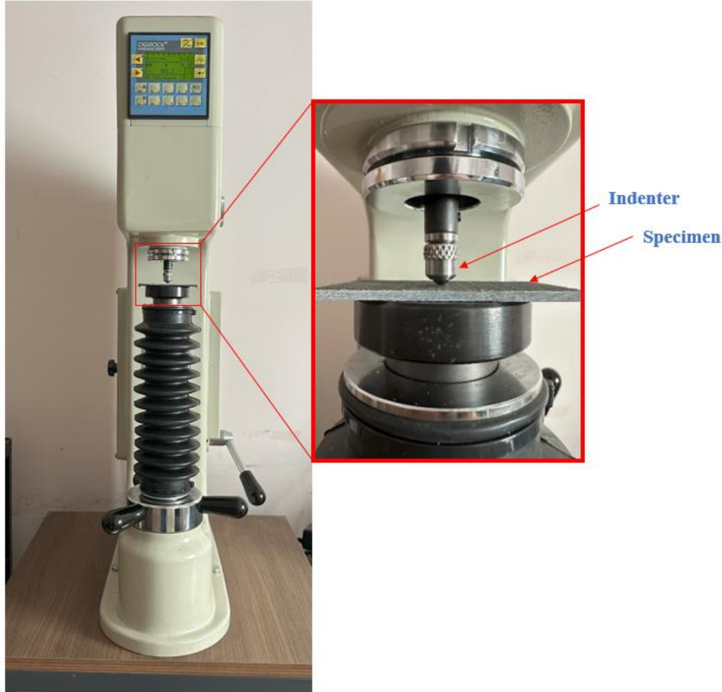
Figure 4. Rockwell hardness test setup for composite specimens (L scale, 6.35 mm steel ball, 10 kg minor load, 60 kg major load)
