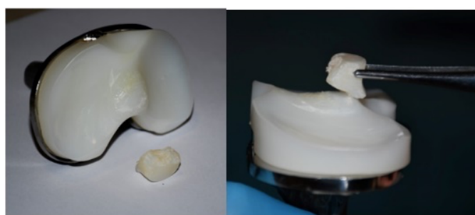
Fig. 3. Macroscopic view of the polyethylene (PE) insert. Visible wear and deformation on the anterolateral aspect of the tibial post are observed, consistent with repetitive cam-post impingement and localized stress concentration
