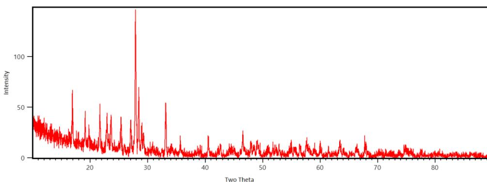
**Figure 1.** The XRD pattern of  $\text{CrVMoO}_7$ .
