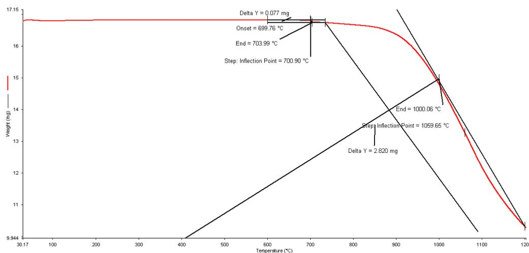
**Figure 6.** TGA thermograph of CrVMoO<sub>7</sub>.
