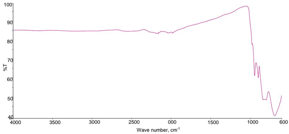
**Figure 3.** The FTIR spectrum of CrVMoO<sub>7</sub>.
