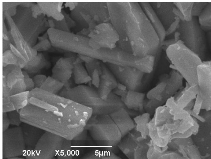
**Figure 4.** The SEM image of CrVMoO<sub>7</sub>.
