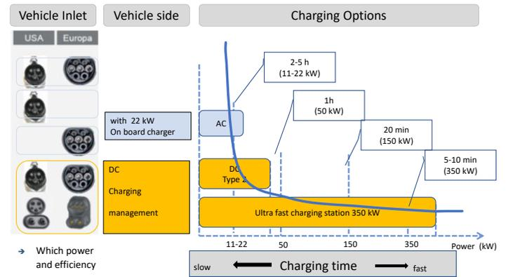
Figure 10. Relationship between charging capacity-charging duration
