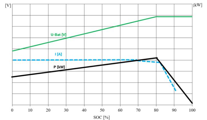
Figure 11. Battery charging power for one charging process
