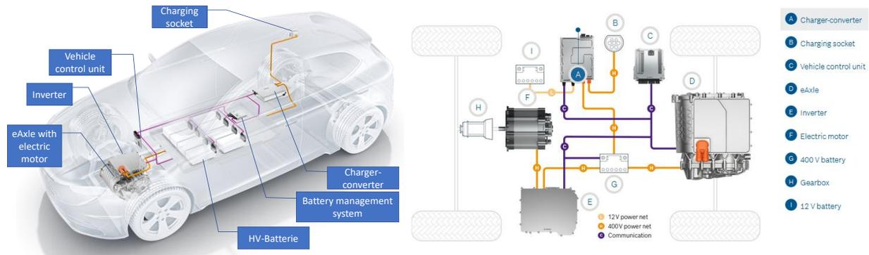
Figure 3. System overview electric vehicle [6]
