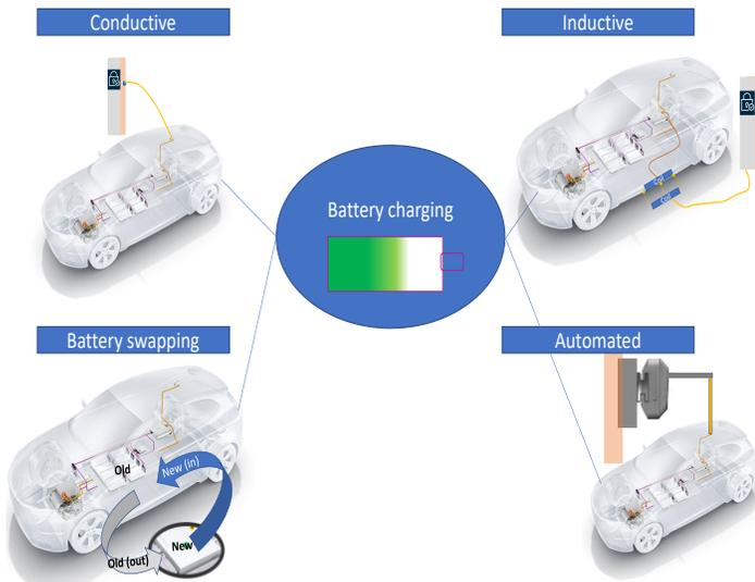
Figure 4. Charging systems for charging the high voltage battery
