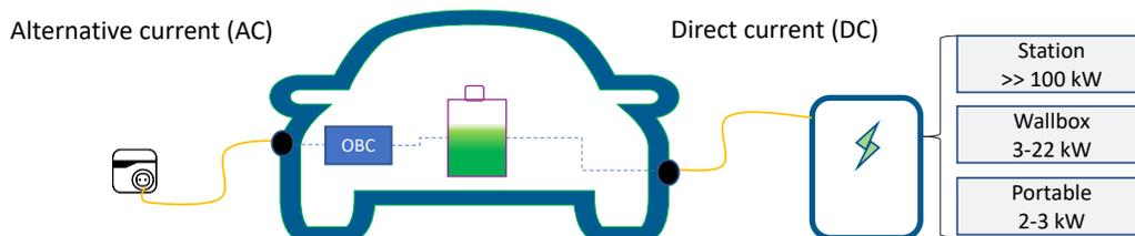
Figure 5. Conductive charging technologies for charging the HV battery
