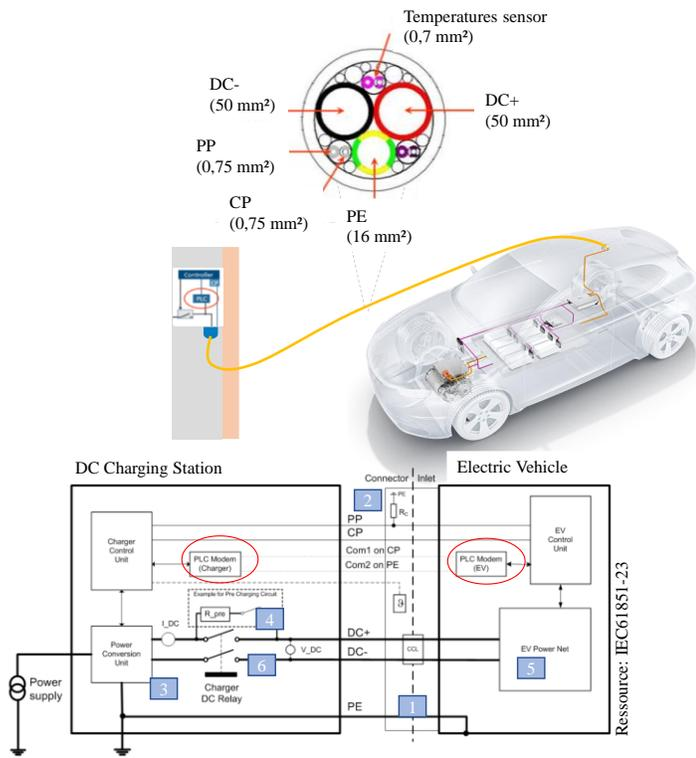
Figure 9. Charging process and architecture for DC charging
