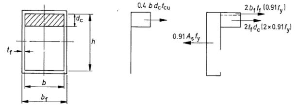
Figure 12. Force diagram for calculating  $M_u$  [32].
