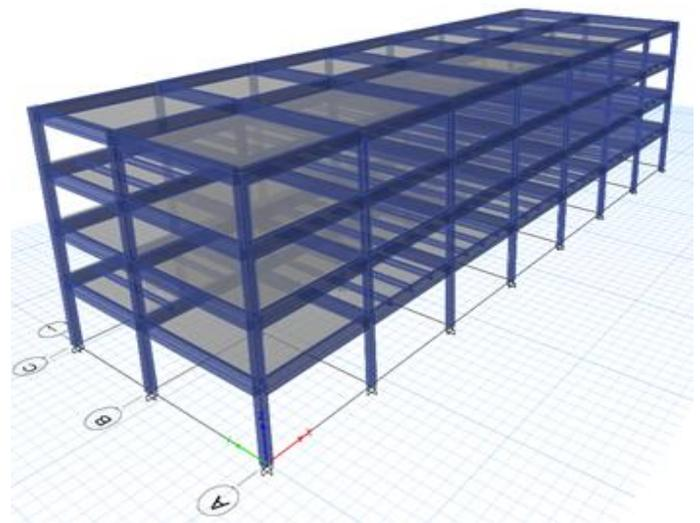
Figure 14. 3D View of the model in ETABS software
