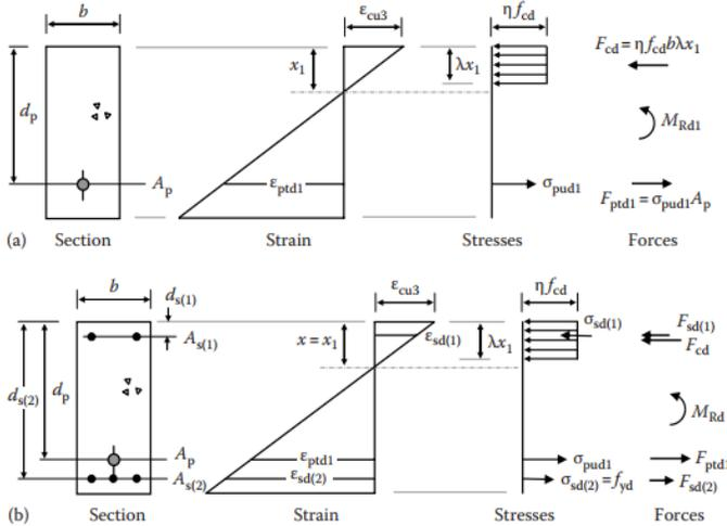
Figure 10, doubly reinforced section [23]
