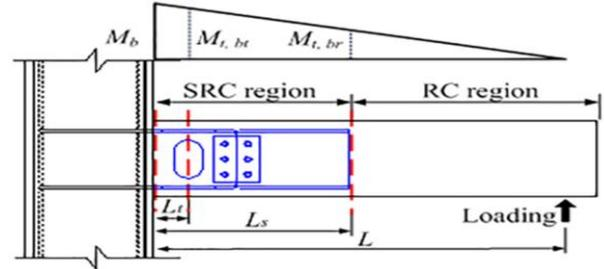
Figure 8. Calculation sketch of hybrid steel precast concrete (HSPC) beam [11].
