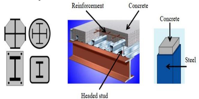
Figure 2. Details of a composite beam, slab and columns [9].
