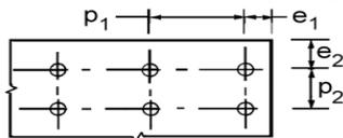
Figure 13. Position of hole for bolts [33].
