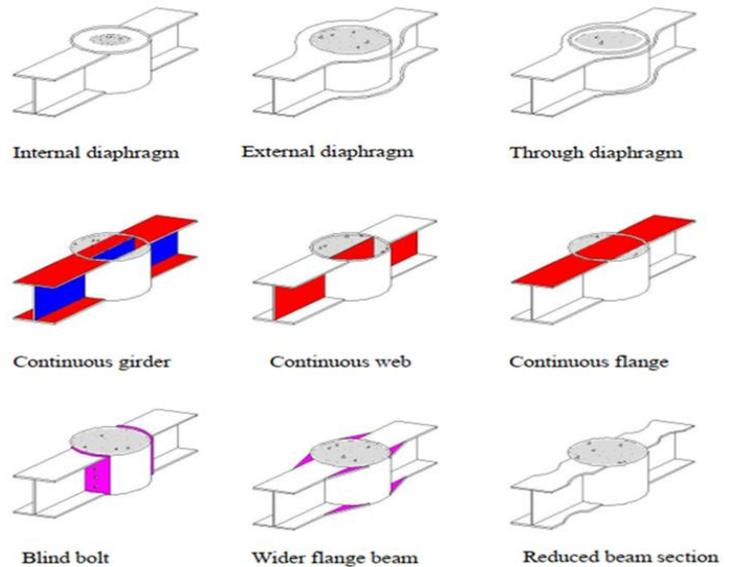
Figure 3. common CFST joint configurations [9].
