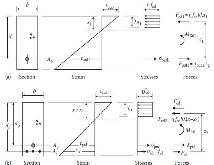
Figure 9. Cross section containing tensile reinforcement [23].
