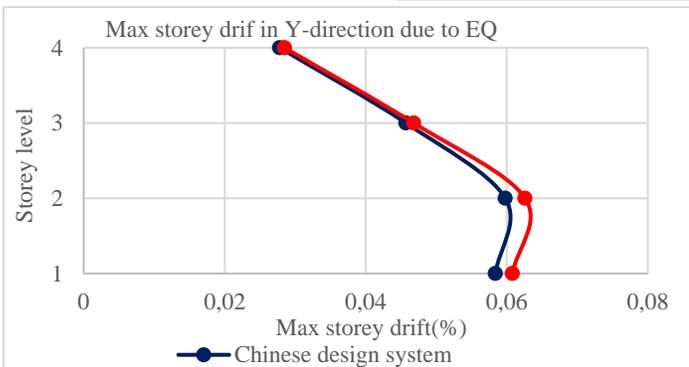
Figure 18. Max interstorey drift in Y-direction due to earthquake
