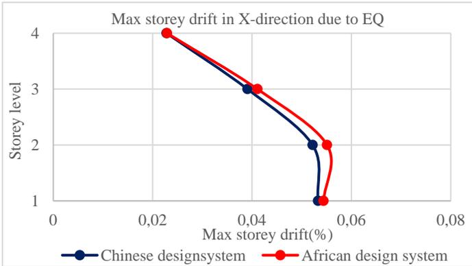
Figure 17. Max interstorey drift in X-direction due to earthquake
