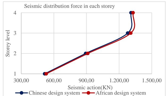
Figure 16. Seismic distribution force in each storey
