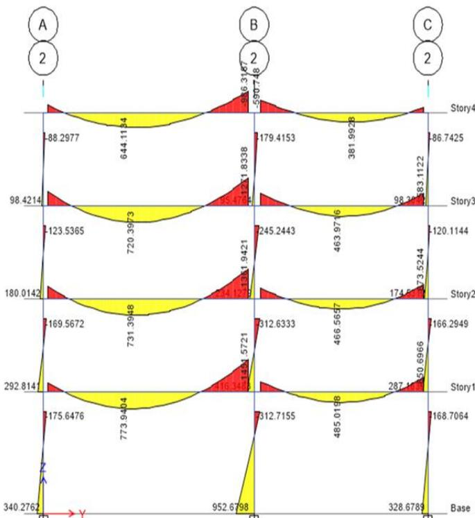
Figure 15. Bending moment diagram
