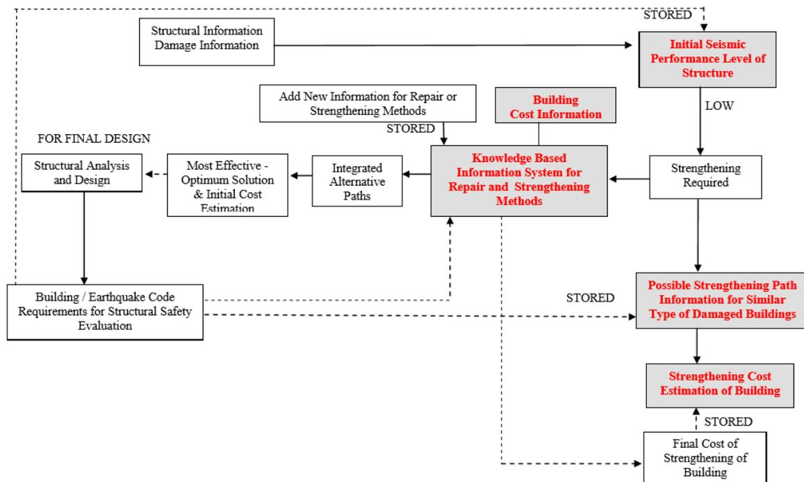
Fig. 6 Evaluation of earthquake damaged building structures
