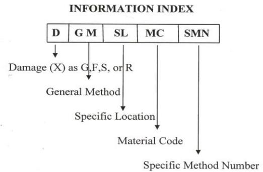
**Fig. 3** Specification of repair methods
