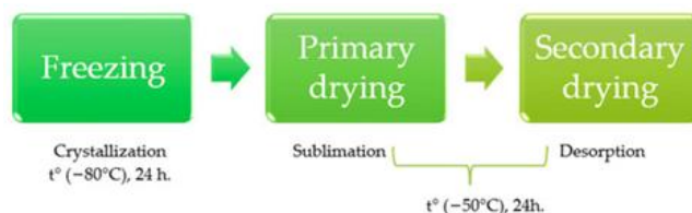
Figure 2. An Outline of the three key steps in the lyophilization process (Stabrauskiene et al., 2024).
