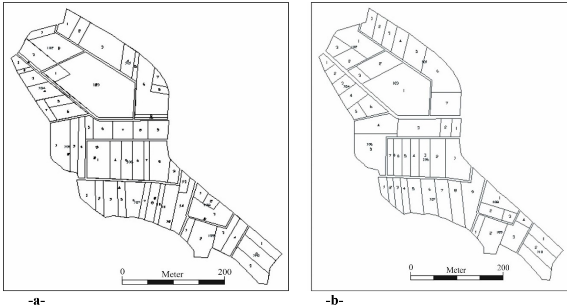
Figure 2. Parcelation plans a) According to the interview-based reallocation model b) According to the block priority-based reallocation model
