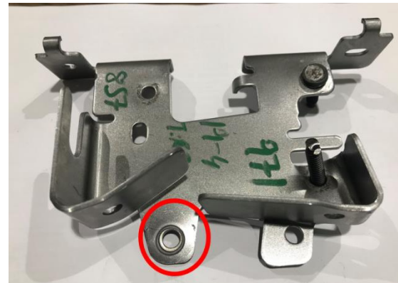
Figure 2. Sheet metal part whose weld bolt falls off due to insufficient weld strength
