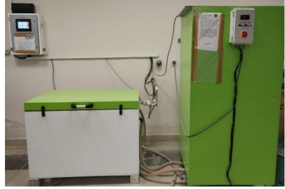
Figure 7. Freeze-thaw test device
