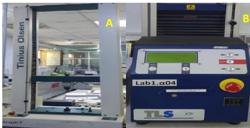
Figure 7. A; Crush tester for bone cement. B; Tensile tester
