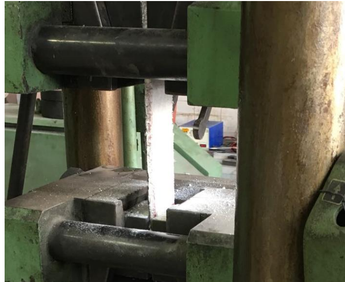
Figure 8. Tensile test applied to the specimens
