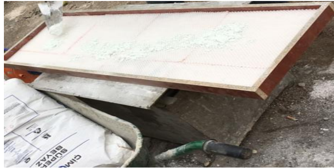
Figure 3. Cement casting into the 3D textile
