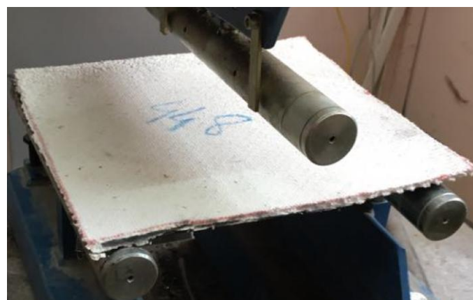
Figure 7. Three-point bending test applied to the specimens
