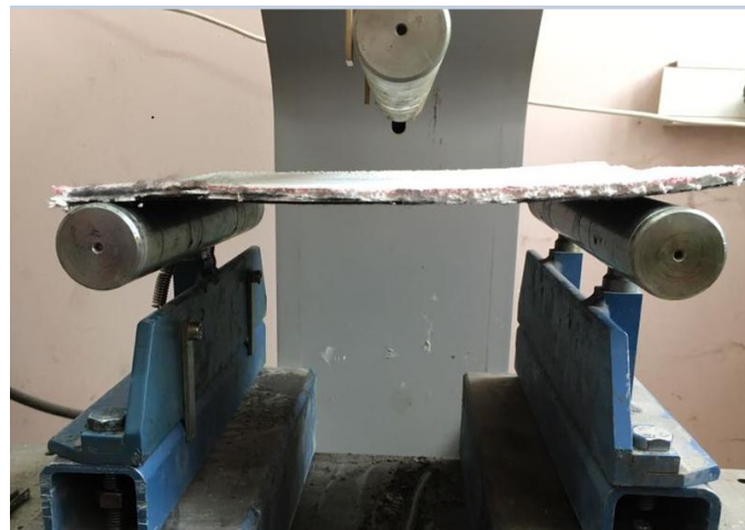
Figure 10. Specimen appearances before the bending test
