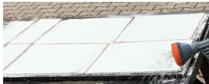
Figure 6. Water immersion of cementitious 3D textile composites
