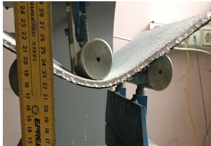
Figure 11. Specimen appearances after the bending test
