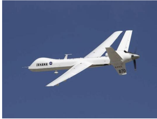
Figure 6. Typical MALE (Medium-Altitude, Long-Endurance) unmanned aerial vehicle (UAV) NASA photograph (2010)
