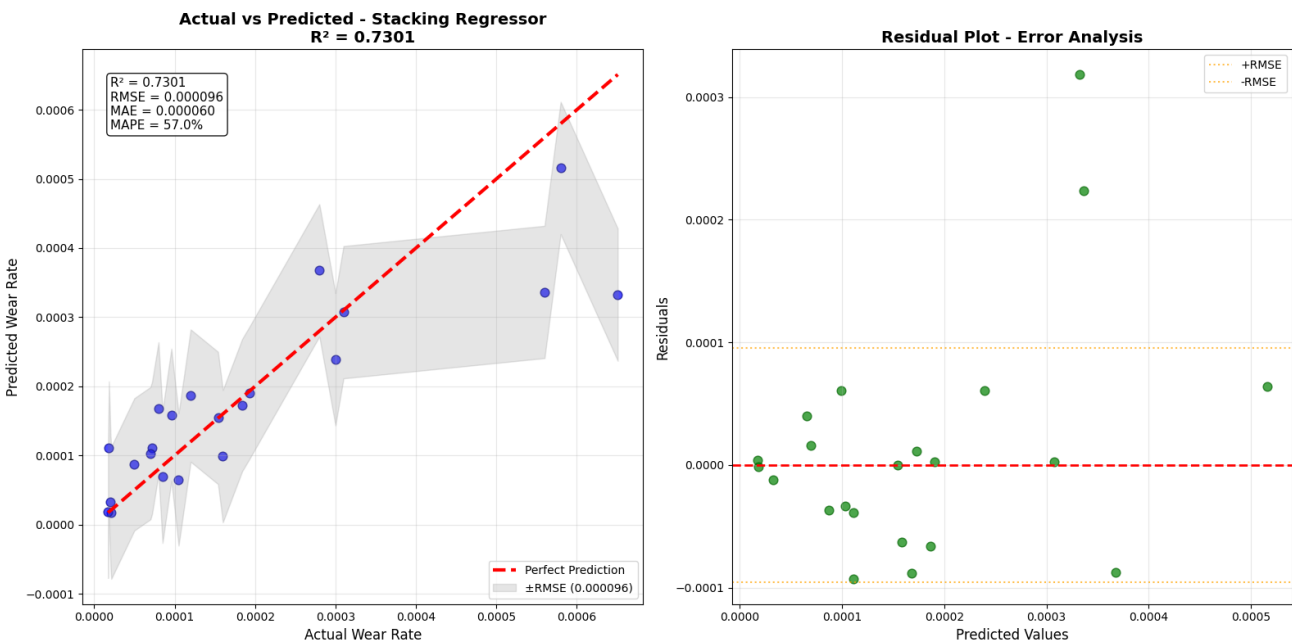
Figure 17: Model validation for wear rate prediction: actual vs predicted values with confidence intervals and residual analysis showing error distribution.
