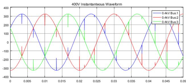
**Figure 11.** Voltage notch waveforms at low voltage bus
