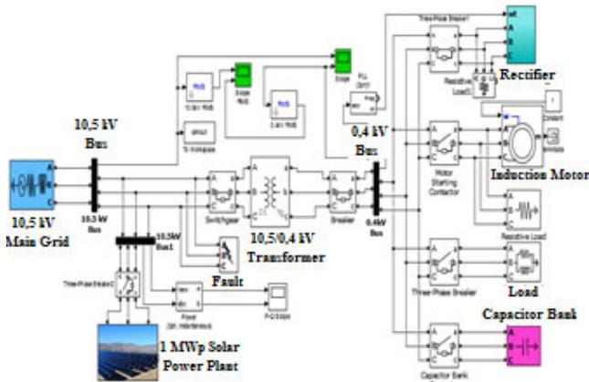
Figure 5. Matlab/Simulink model of the developed electrical power distribution system
