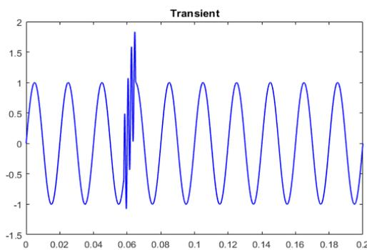
**Figure 3.** Transient disturbances waveform
