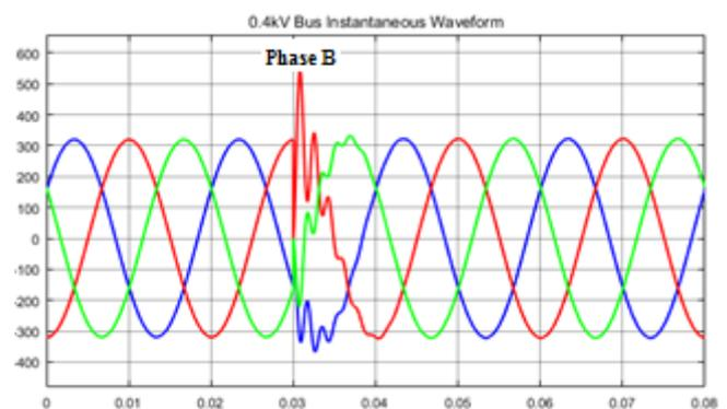
**Figure 10.** The voltage waveforms resulting from the switching of the capacitor bank
