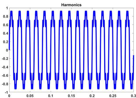
Figure 2. Harmonics caused by universal bridge connection
