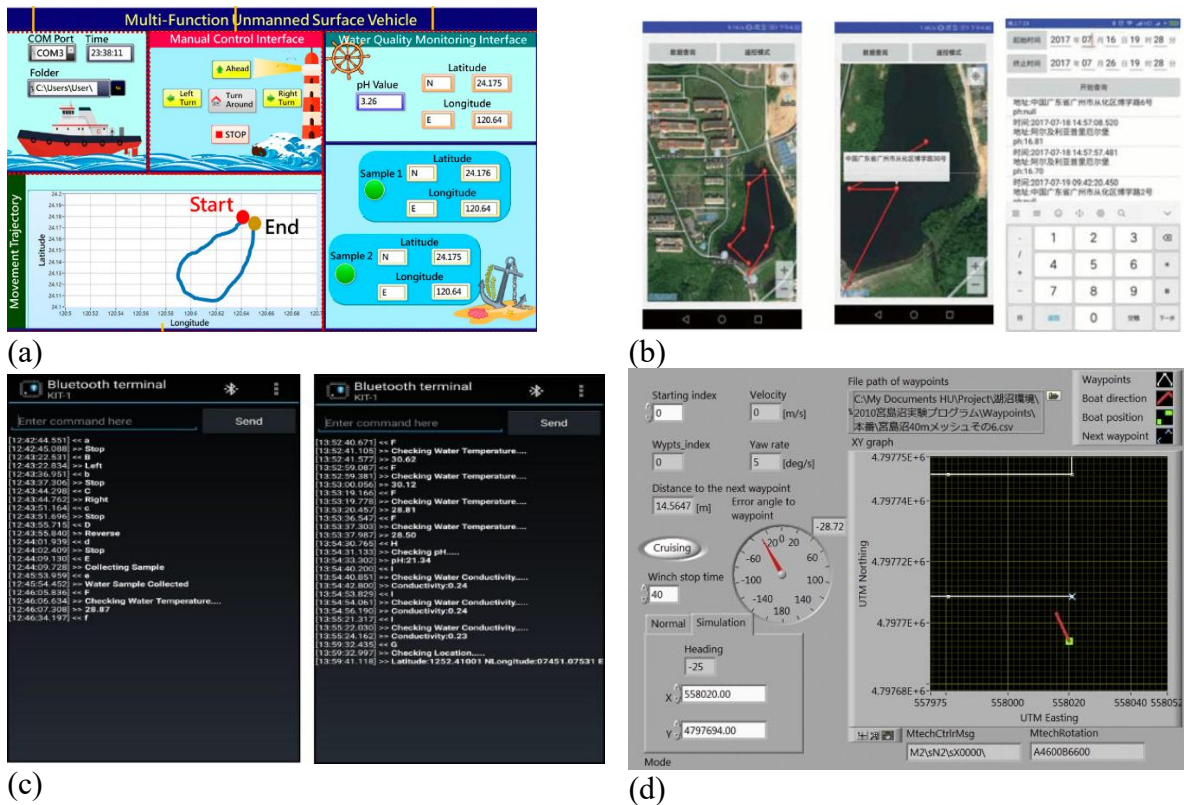
Figure 4. (a) Control unit developed using LabVIEW (Chang et al., 2021), (b) Control unit developed with a mobile application (Cao et al., 2018), (c) Mobile application with text-based command input (Dsouza et al., 2021), (d) Computer-based control unit (Kaizu et al., 2011)
