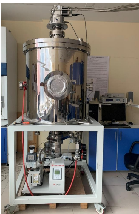
Figure 2. Low-temperature magnetic levitation force measurement system (MLFMS)
