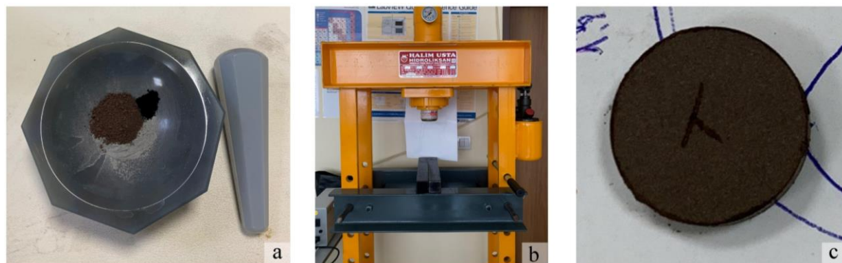
Figure 1. Preparation process of \text{MgB}_2 -PAni bulk samples: (a) mixing precursor powders in an agate mortar, (b) pressing under 2 bar to form pellets, and (c) final pellet shape before heat treatment
