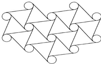
Figure 11. Auxetic 2D asymmetric hexagonal model [31]
