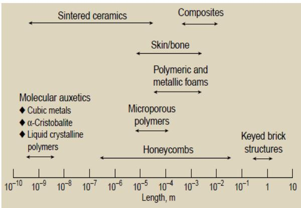
Figure 2. Auxetic structures and materials in various levels [4]
