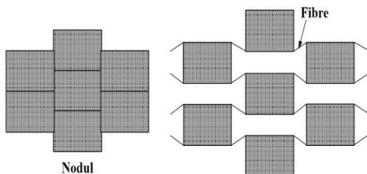
Figure 7. 2-dimensional model of auxetic ePTFE [25]
