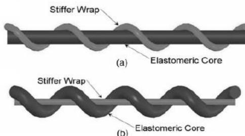
Figure 16. Structure of auxetic helical yarn in (a) unstretched, (b) stretched status [60]
