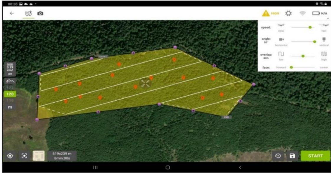
Figure 3. UAV flight line and photo location, red points represent the sample plot centers where field measurements were conducted, the black polygon represents the boundary of the flight, and the white lines represent the path followed by the UAVs during the image capture phase
