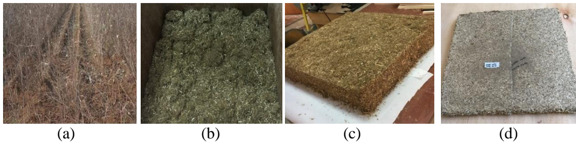
Figure 1. Production stages of test samples: a)-In the field, b)-Chipping, c)-Pressing, d)-Sample
