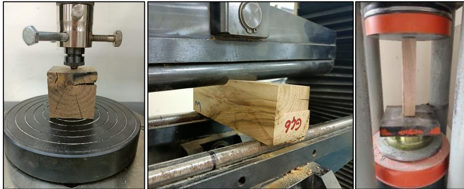
Figure 2. Mechanical tests applied to the specimens, from left to right: brinell hardness test, three-point bending test and compression test parallel to the grain
