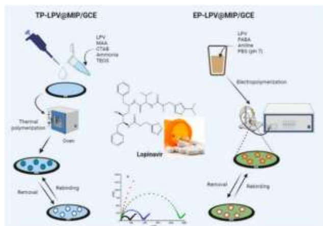
Figure 2. Schematic diagram of the molecular imprinted sensor design for LOP. Reprinted from Faysal et al. 39 with permission from Elsevier
