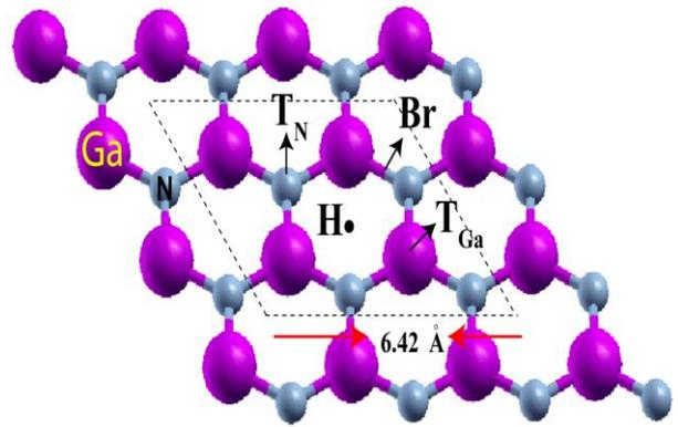
**Figure 1.** h-GaN monolayer.  $(2 \times 2)$  GaN supercell with lattice constants  $a=b=6.42$  Å is delineated by dashed lines. Possible adsorption sites are also illustrated.
