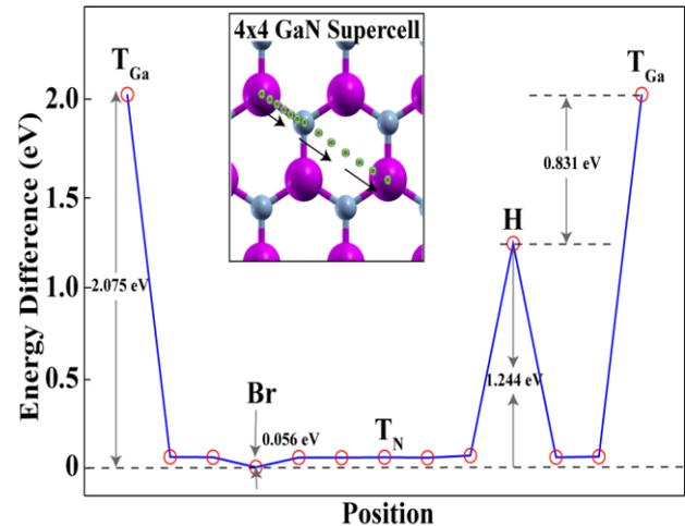
**Figure 3.** Diffusion of Pt atom on (4×4) GaN monolayer. Green dots show Pt position on GaN and arrows show the diffusion path.
