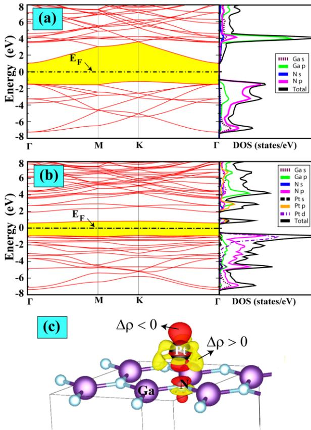
**Figure 2.** (a) Electronic band structure of bare (2×2) GaN monolayer, the electronic partial density of states are given in the right panel. (b) Electronic band structure of Pt adsorbed (2×2) GaN monolayer for the most favorable configuration, the electronic partial density of states are given in the right panel. (c) Charge density isosurfaces are shown. Red depicts the depletion of charge, while yellow is for accumulation.
