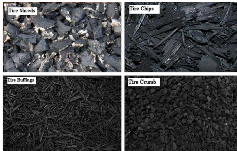
Figure1. Typical shapes of different processed tire wastes (not to scale) (Edinçliler et al. 2010).
