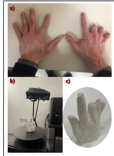
Figure 1(a): Hands of the amputee. (b): Scanning of the plaster model. (c): Plaster model of the partial hand amputee.
