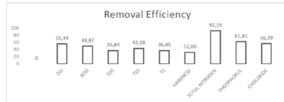
Figure 6: Chart showing the percentage removal efficiency of the filter media
