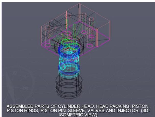
Fig. 3. CAD Model (Wireframe) of piston, cylinder head and cylinder sleeve assembly
