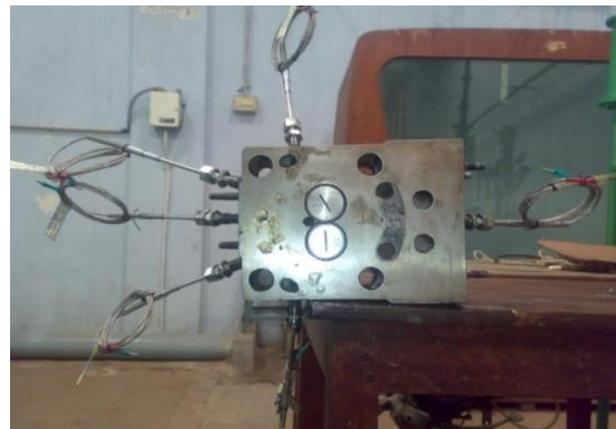
Fig. 5. Cylinder Head with fitted thermocouples
