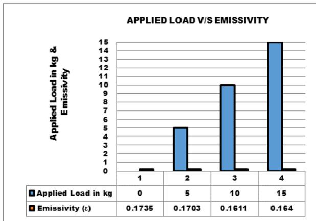
Fig. 16. Variation of emissivity values at various applied loads
