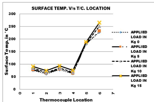
Fig. 8. Measured Temperature Values at different loads 0 kg, 5 kg, 10 kg and 15 kg
