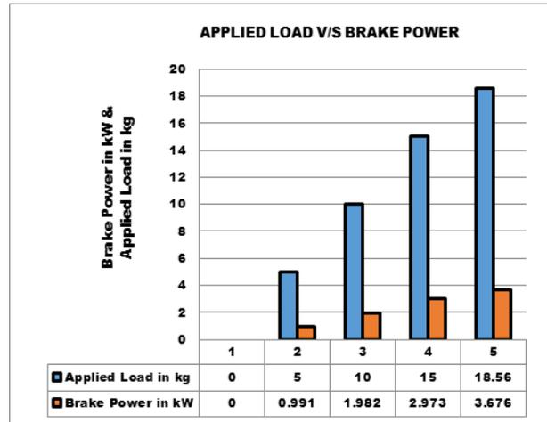
Fig. 11. Variation of brake power at various applied loads
