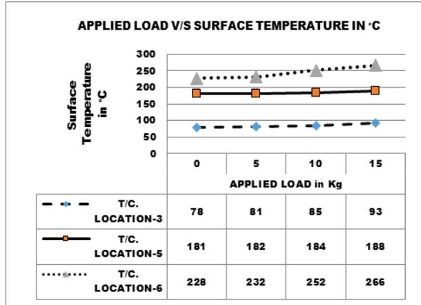
Fig. 10. Measured temperature values from thermocouple locations-3, 5 and 6 for different applied loads of 0 kg, 5 kg, 10 kg and 15 kg
