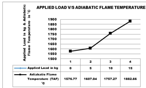
Fig. 12. Variation of adiabatic flame temperature values at various applied loads
