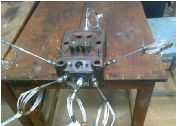
Fig. 6. Cylinder Head with fitted thermocouples
