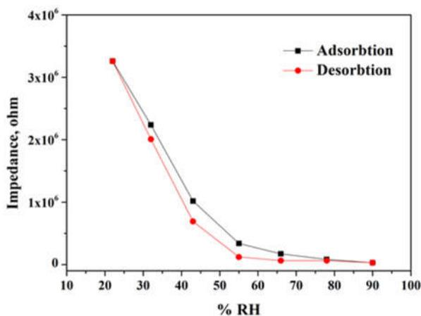
Figure 5. Humidity Hysteresis loop of the Co-Mg sample.
