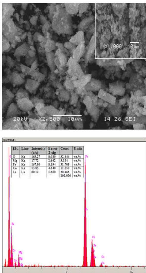
Figure 2. SEM micrographs at different magnitude and EDX analysis of Co-Mg ferrite nanoparticle
