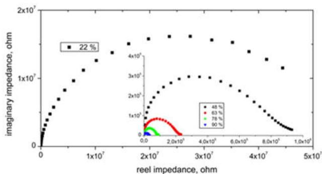
Figure 8. Co-Mg ferrites impedance measurement for Argand diagram.
