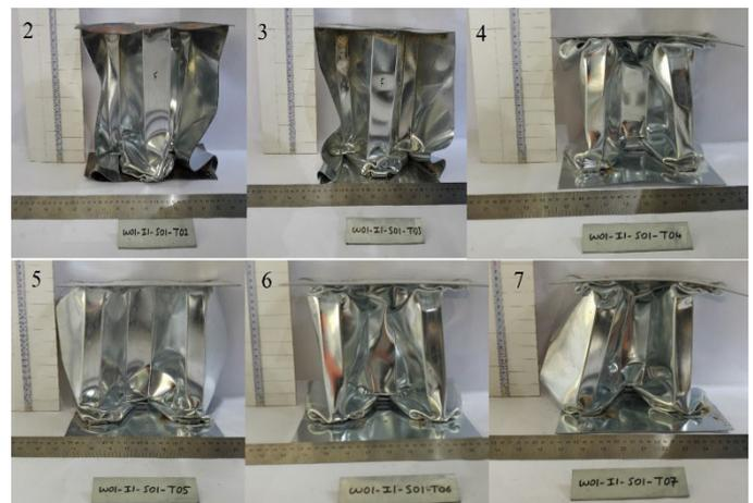
Figure 7. Drop test results of the 1mm thick specimen
