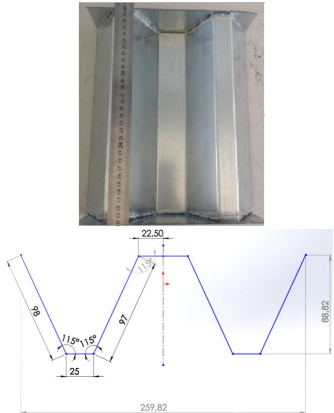
**Figure 3. Dimensions of the W cross section**
