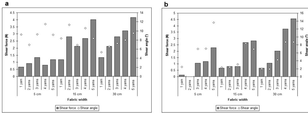
**Figure 6.** Relationship between shear force-angle and the number of pulled ends for various fabric widths in dry polyester fabric a) Pulled direction: warp, b) Pulled direction: weft (Fabric length: 20 cm).
