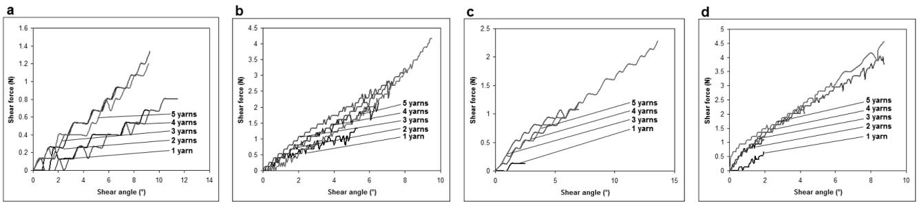
**Figure 3.** Shear force-angle curves of untreated polyester ribs fabrics. a) Pulled ends:1-5, pulled direction: warp, fabric width: 5 cm, fabric length: 20 cm. b) Pulled ends:1-5, pulled direction: warp, fabric width: 30 cm, fabric length: 20 cm. c) Pulled ends:1-5, pulled direction: weft, fabric width: 5 cm, fabric length: 20 cm. d) Pulled ends:1-5, pulled direction: weft, fabric width: 30 cm, fabric length: 20 cm.
