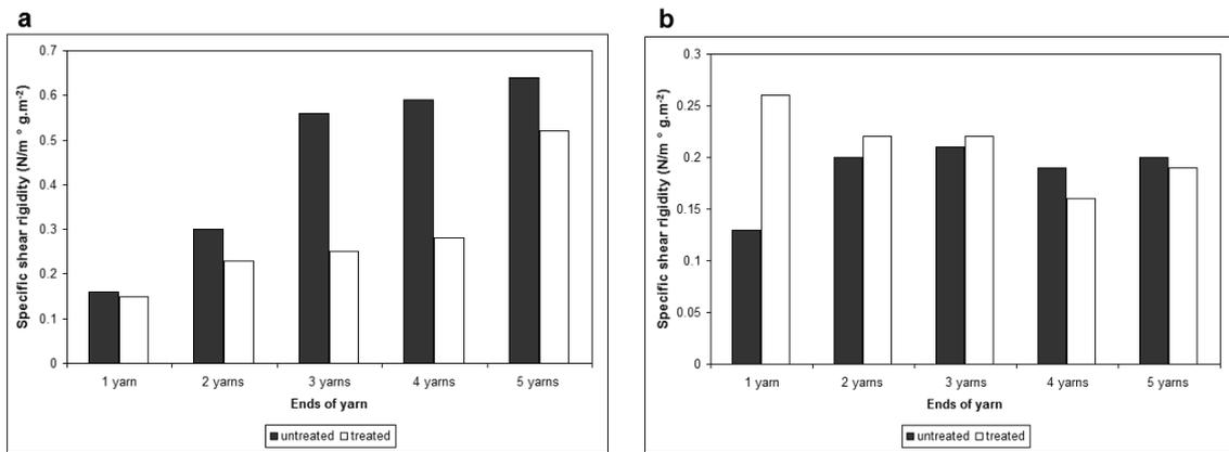
**Figure 12.** Relationship between specific shear rigidity and the number of pulled ends for various fabric width/length ratios in untreated and softening agent treated polyester ribs fabric a) Pulled direction: warp, b) Pulled direction: weft (Fabric width: 30 cm, fabric length: 10 cm, fabric width/length ratio:3/1).
