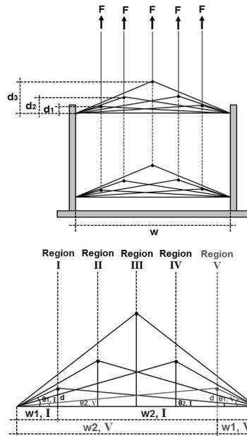
**Figure 8.** Schematic view of pull-out yarn end positions from different regions of woven fabric during pull-out test to find fabric local shear (left) and top portion of various regional shear displacements and angles (right).
