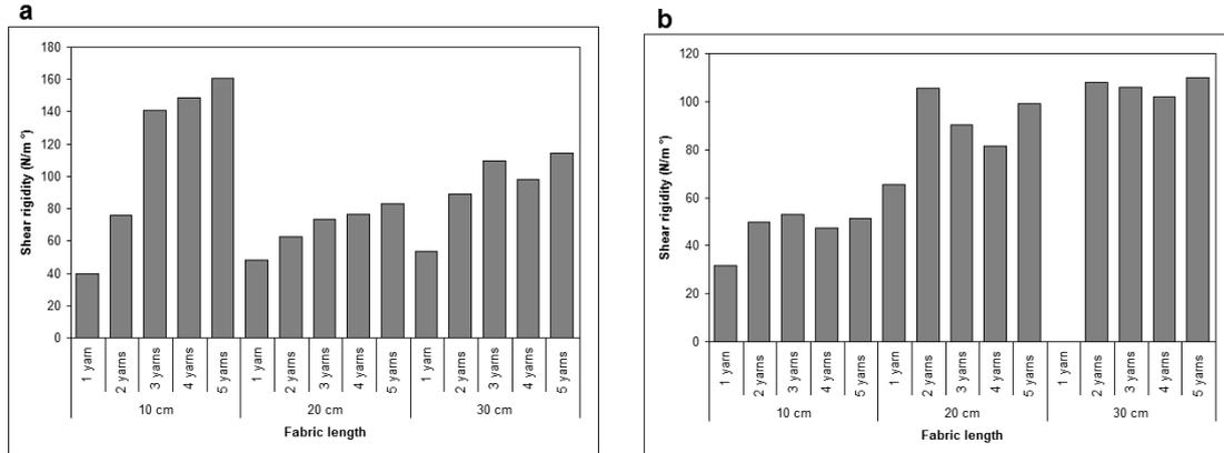
Figure 9. Relationship between shear rigidity and the number of pulled ends for various fabric lengths in untreated polyester ribs woven fabric a) Pulled direction: warp, b) Pulled direction: weft, (Fabric width: 30 cm).
