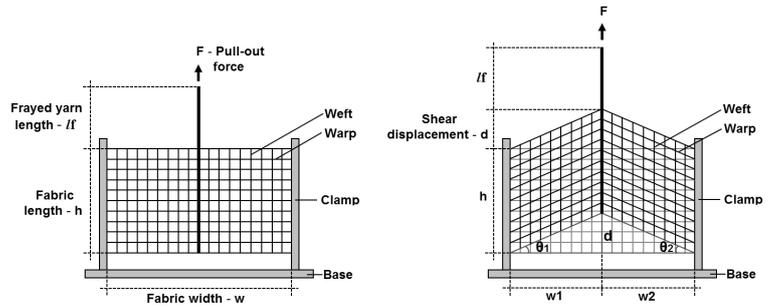
**Figure 1.** Pull-out fixture with fabric sample on the tensile testing instrument (left), schematic views of the fabric and yarn pulled-ends for fabric shear by pull-out test; Initial fabric position before fabric shear by pull-out test (middle), fabric shear before crimp extension starts (right).
