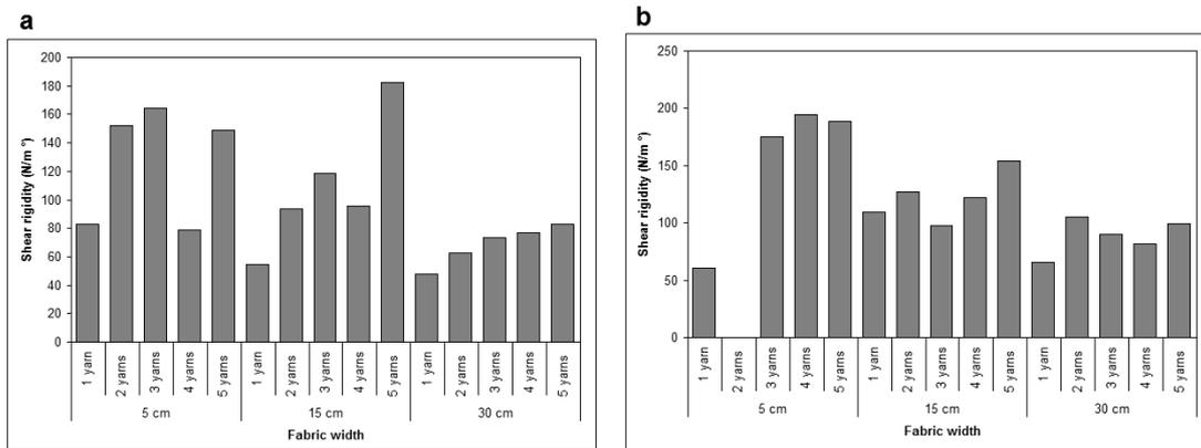
Figure 10. Relationship between shear rigidity and the number of pulled ends for various fabric widths in untreated polyester ribs woven fabric a) Pulled direction: warp, b) Pulled direction: weft, (Fabric length: 20 cm).
