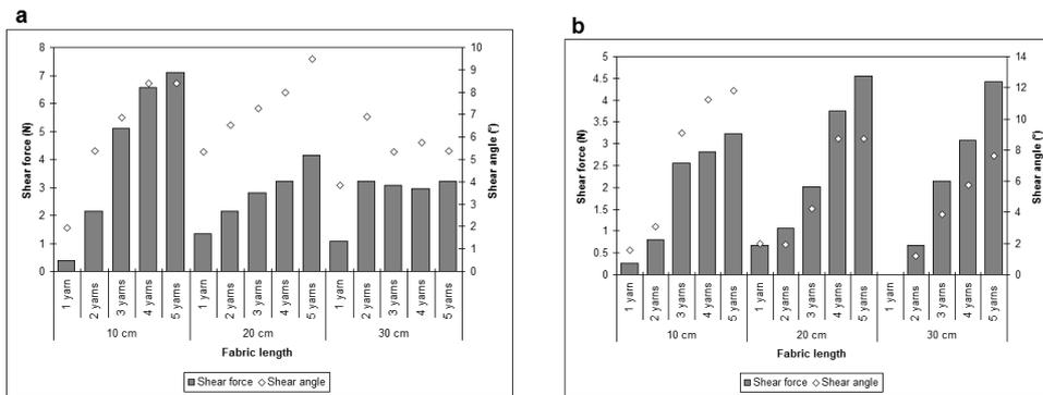
**Figure 5.** Relationship between shear force-angle and the number of pulled ends for various fabric lengths in dry polyester fabric a) Pulled direction: warp, b) Pulled direction: weft (Fabric width: 30 cm).
