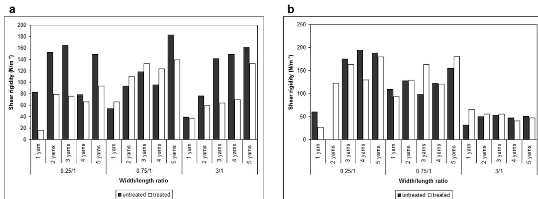
Figure 11. Relationship between shear rigidity and the number of pulled ends for various fabric width/length ratios in untreated and softening agent treated polyester ribs fabric a) Pulled direction: warp, b) Pulled direction: weft.
