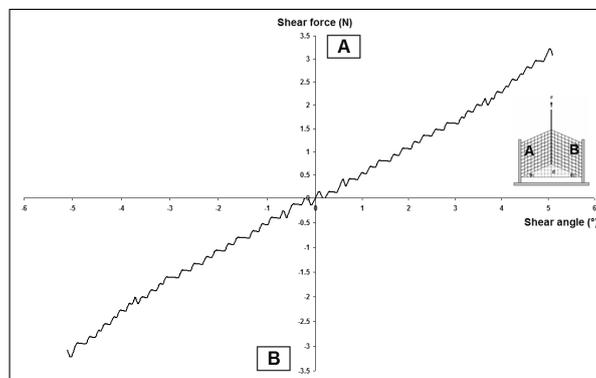
**Figure 2.** Woven fabric shear force-angle curve in warp direction of fabric part A and B before crimp extension stage. (Fabric; Polyester dry fabric, Pulled ends; 5 yarns, Fabric width and length; 30 x 30 cm.)
