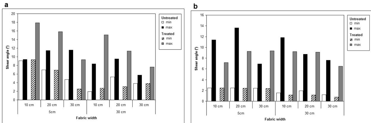
**Figure 13.** Shear angle jamming for various fabric widths and lengths in untreated and softening agent treated polyester ribs fabrics a) Pulled direction: warp, b) Pulled direction: weft.
