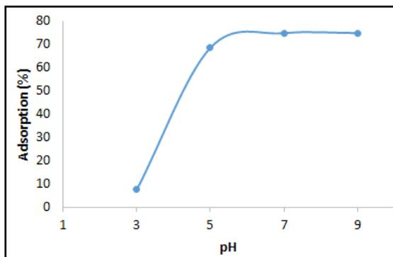
Fig 2. Adsorption percentage of Cu (II) ions for different pH values
