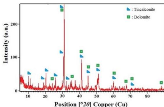
Fig 1. XRD pattern of borax sludge [18]
