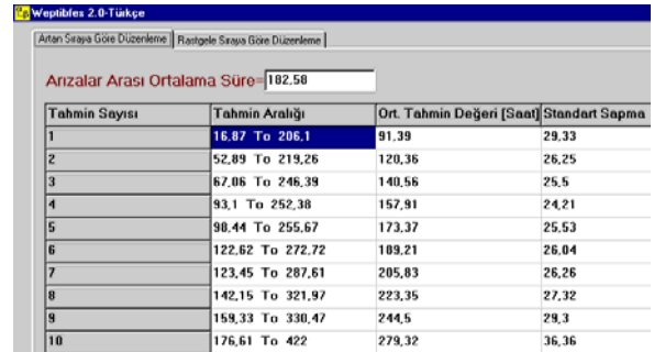
Figure 10. Results Screen for Monte-Carlo simulation according to WEIBULL distribution parameters calculated by failure data of General Motion Transmission Elements.
