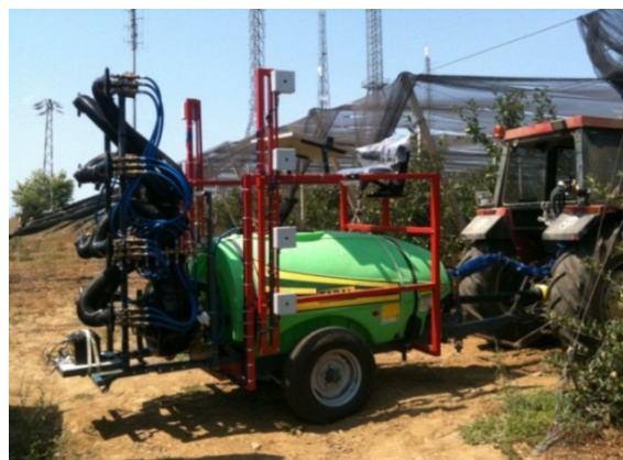
Figure 1. A prototype sprayer during the experiment in the orchard;
