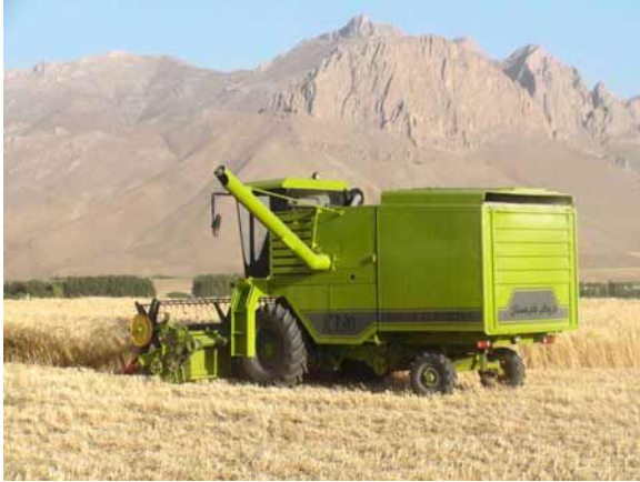
Figure 2. Modified combine with straw container to collecting the straw.
