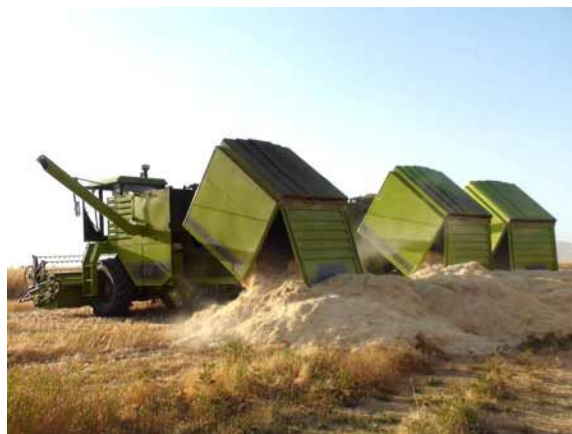
Figure 1. The modified wheat harvesting combine
