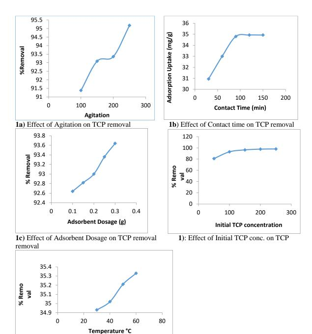
**1e**) Effect of Temperature on TCP removal **Figure 1(a – e).** Effect of Adsorption factors on TCP removal
