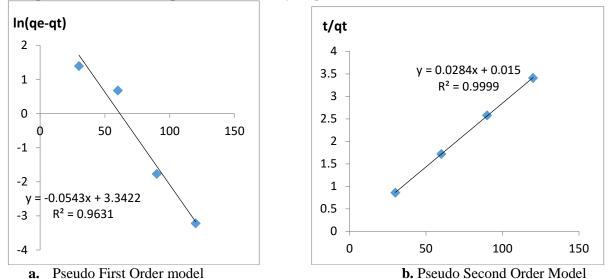
Figure 3. Plots of Kinetic Models for Adsorption of TCP onto FPBAC
