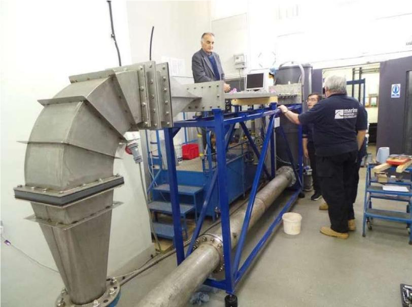
**Fig. 2.** A view of new test section of the UNEW Flow Cell
