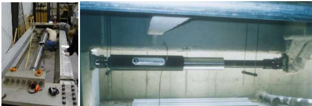
Fig.10. Steel Dampers: These dampers without a capacity of vertical load bearing are often used with elastomeric bearings. With these systems used commonly in Japan, earthquake energy is absorbed.
