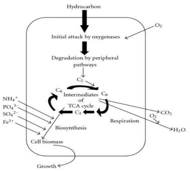
**Figure 1**. Main principle of aerobic degradation of hydrocarbons by microorganisms (Chaillan et al,. 2006).
