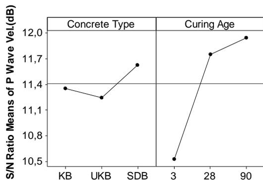
Figure 2. Main effects plot of P wave velocity for S/N ratios
