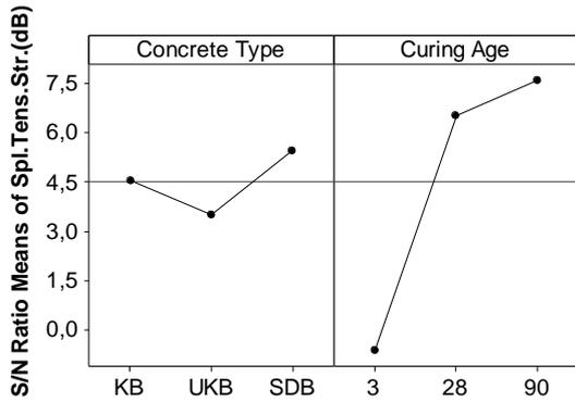
Figure 4. Main effects plot of splitting tensile strength for S/N ratios
