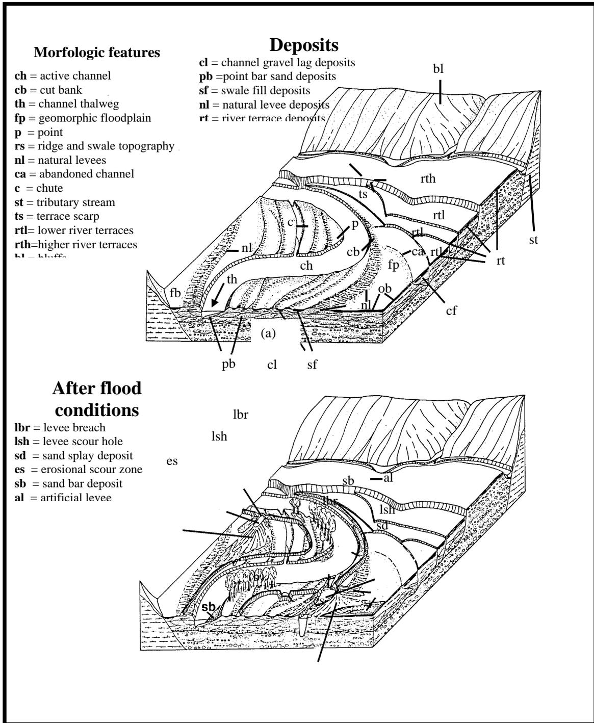
Figure 4. (a) Natural morphologic features and conceptual floodplain stratigraphy of the Missouri River, (b) after flood condition of the flood plain. During 1993 flood, the floodplain inundated bluff to bluff (SAST, 1994).
