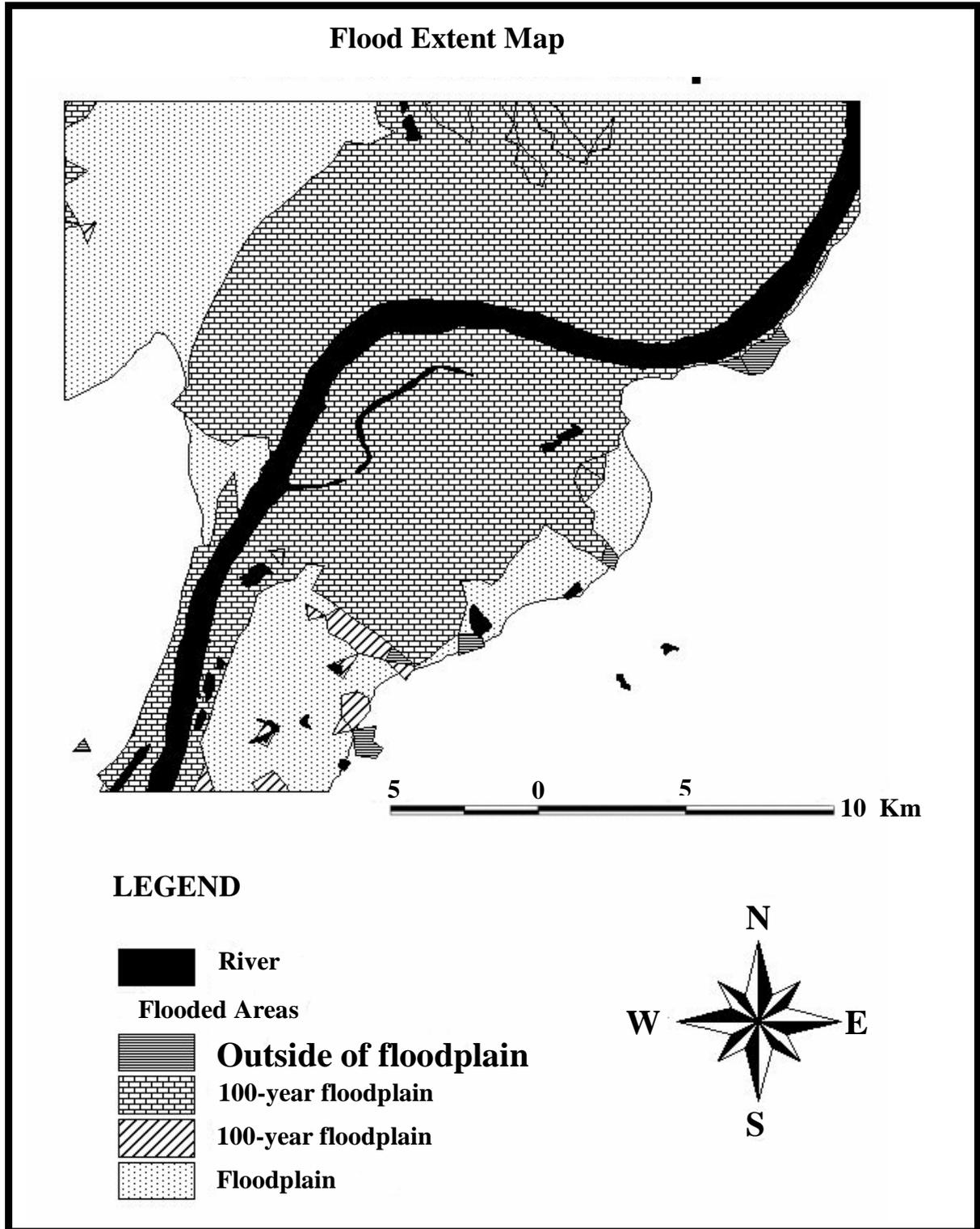
Figure 7. Flooded areas in 1993 (Flood Classification). Most of the floodplain areas were covered by 100-year flood which caused severe damages along the river.
