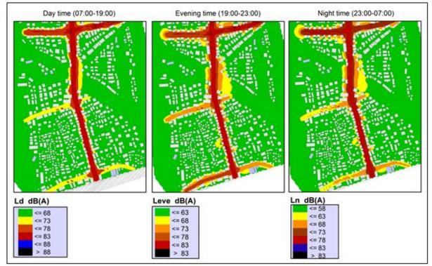
Figure 4. Noise distribution maps of Bulent Angin Boulevard according to Regulation on Environmental Noise Assessment and Management
