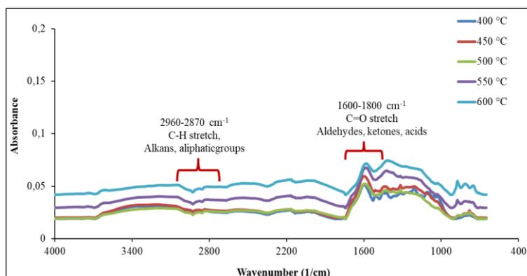
Fig 3. FT-IR spectra of bio-char samples
